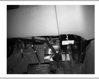
FT1 mounted under dash using OBDII T Harness cable & tie straps to securely fasten device to chassis of vehicle
